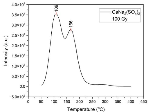
Figure 18: TL glow curve of  $\text{CaNa}_2(\text{SO}_4)_2$  for 100 Gy gamma radiation
