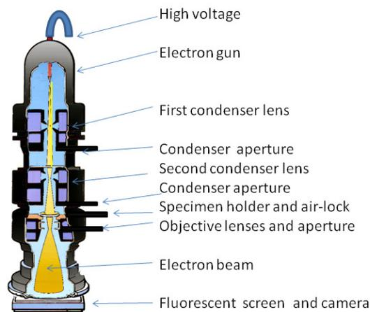
Figure 5: Transmission Electron Microscope
