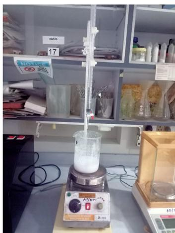
Figure 9: Formation of precipitate due to drop-wise addition of  $(NH_4)_2SO_4$  to the solution
