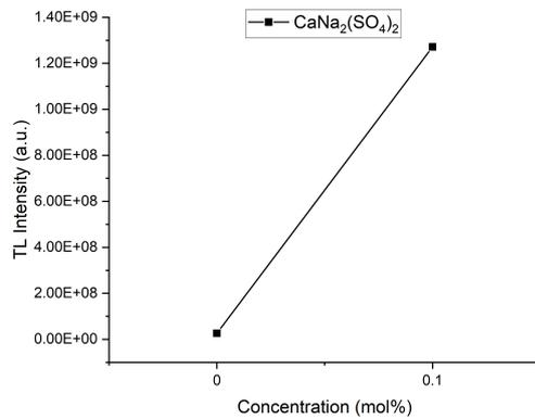
Figure 17: Intensity vs dopant concentration for 50Gy gamma radiation
