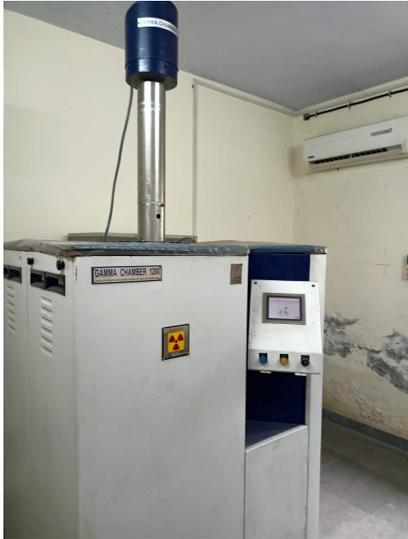
Figure 15: Gamma Ray irradiation chamber
