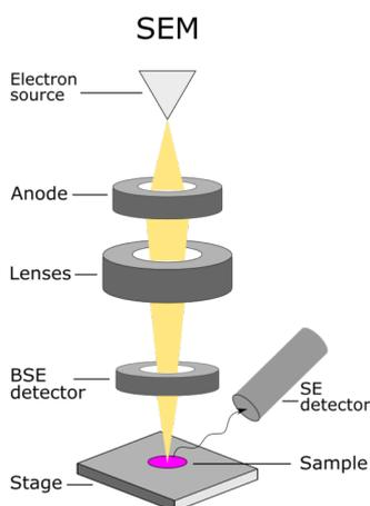
Figure 6: Scanning Electron Microscope
