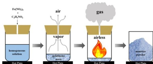
Figure 4: combustion method
