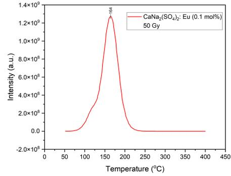
Figure 19: TL glow curve of  $CaNa_2(SO_4)_2$  for 50 Gy gamma radiation      Figure 20: TL glow curve of  $CaNa_2(SO_4)_2 : Eu(0.1mol\%)$  for 50 Gy gamma radiation
