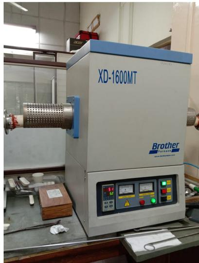
Figure 14: Muffle Furnace for annealing the sample
